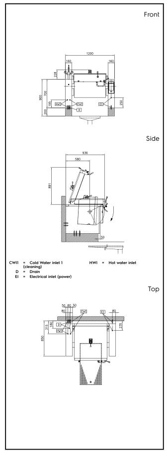
Electric 400 V/3N ph/50/60 Hz Supply voltage: Total Watts: 15.5 kW Installation: FS on concrete base;FS on feet;On base;Standing Type of installation: against wall
